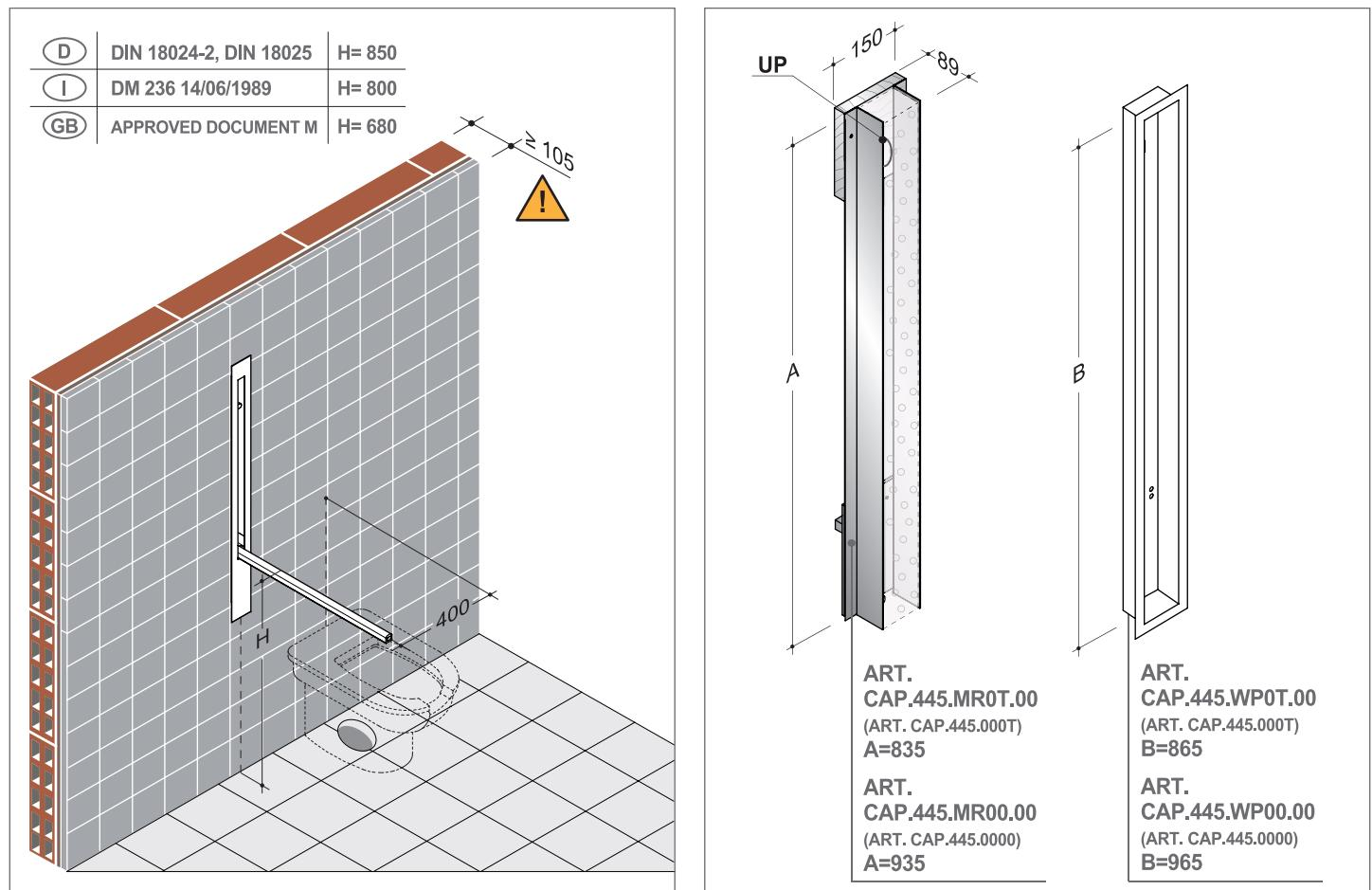
PROCEDURA DI INSTALLAZIONE - INSTALLATION PROCEDURE - PROCEDURE D'INSTALLATION - INSTALLATIONSVERFAHREN - PROCEDIMIENTO DE INSTALACION - INSTALLATIEPROCEDURE
